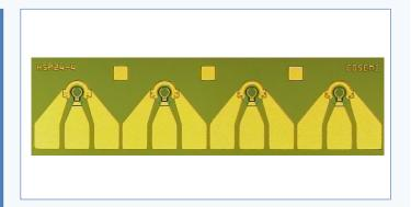
Cosemi's LPD3025-4 is a mesa-structured, InGaAs-based PIN photodiode 1x4 array offering high responsivity, low dark current and low capacitance for high bandwidth, high performance optical receiver designs.
